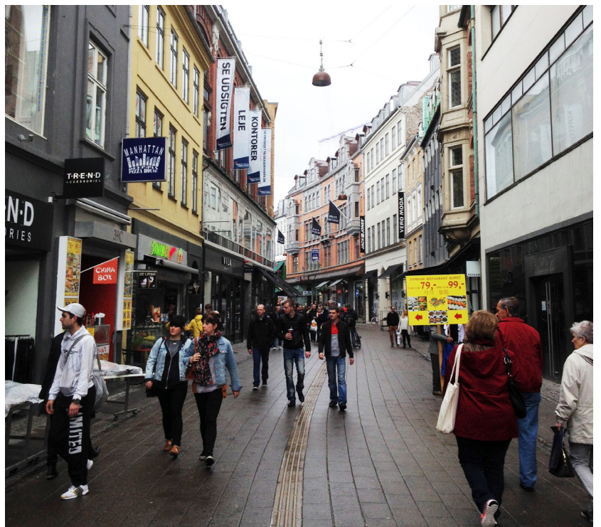
Fig 3.1b Tactile indicators when used effectively can enhance the footpath and help people with visual impairment.
