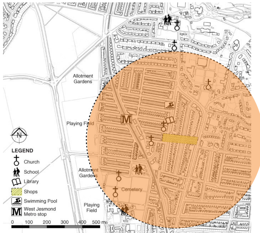
Fig 1.1 500m radius walking circle (about a 10 minute walk). The yellow represents the shopping centre catchment. Note that nearly all the denser housing is within this 500m radius; that there are different uses; and the slightly irregular grid pattern.
