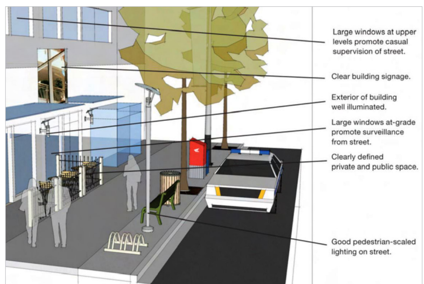
Fig 1.2b A diagram illustrating some CPTED principles; passive surveillance and lighting are simple, non intrusive ways to improve safety and security. From metrolix.com Mobility Hub Guidelines.
