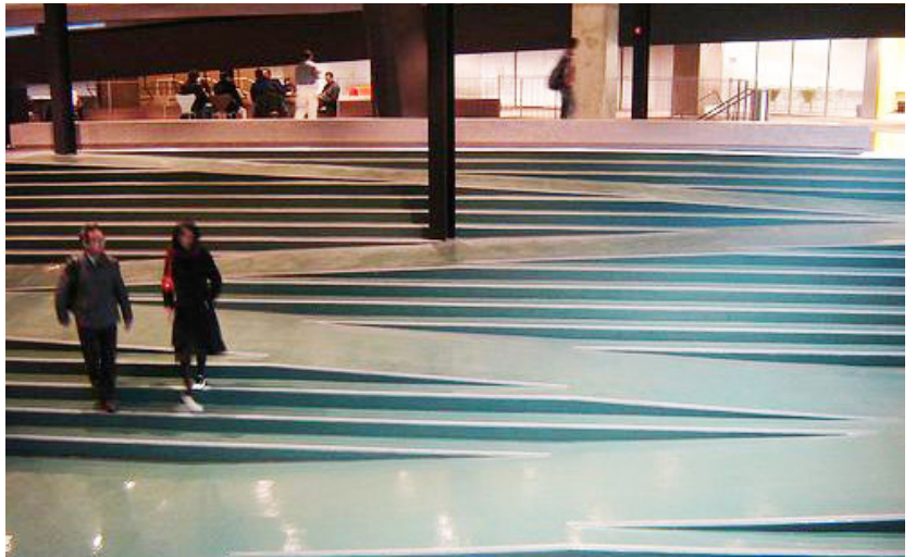
Fig 3.2b Some ramps may not strictly comply with access code requirements but can still highlight inclusiveness and provide an alternative to stairs.
