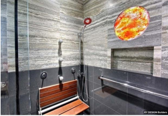
Figure 16: In order to produce an adaptable space for the proposed model's shower, a fold up bench would be recommended to be installed instead of built-in bench. Source: http://www.houzz.com/ideabooks/1061289/list/Bathroom-Safety-Features-That-Support-Your-Style
