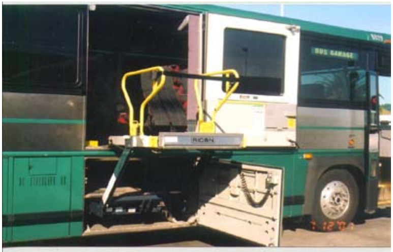
Figure 4.6. An over the road bus, with a lift deployed.
