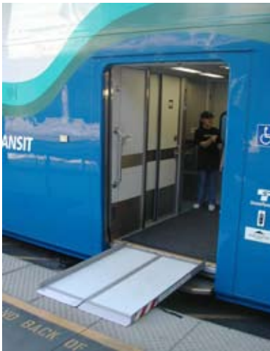
Figure 4.3. Bi-level vehicle with bridge ramp (Source: Paul Ryus)
