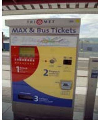
Figure 4.4. Trimeter's ticket machine is color coded for each step in the process (Source: Paul Ryus).
