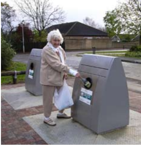
Figure 6.5. Waste receptacles with main containers in shafts
